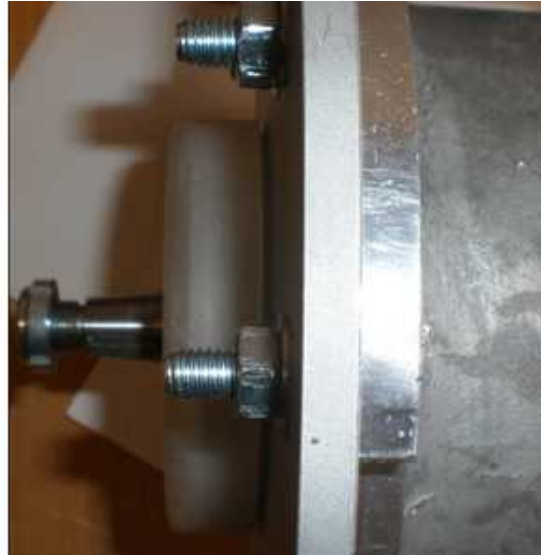
Figure 19: Back flang mounted and detail of the screw with lock washers.
