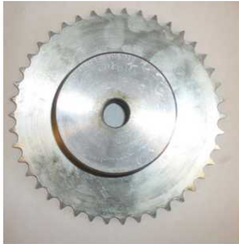
Figure 27: New free toothed wheel before manufacturing
