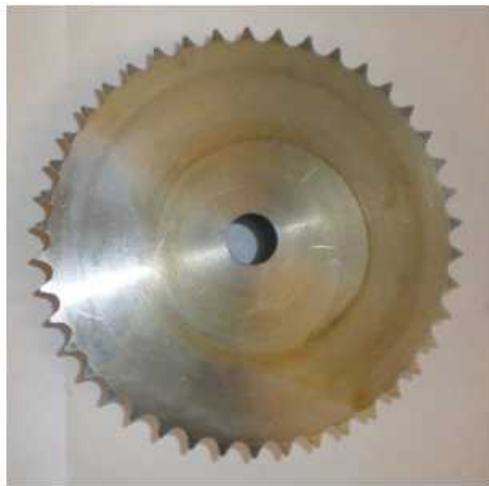
Figure 27: New free toothed wheel before manufacturing
