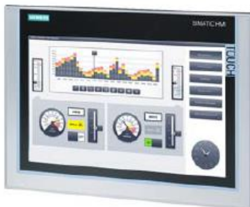
Fig. 68 HMI TP1200 Comfort
