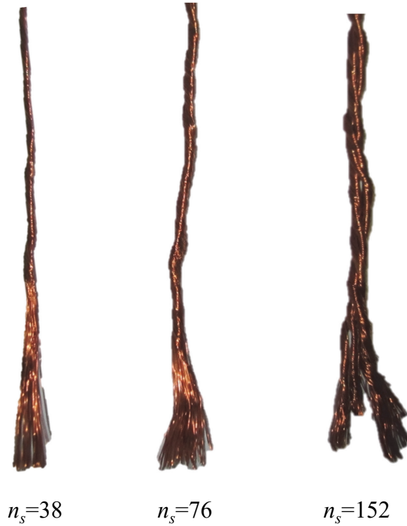
Figure B.1: Litz wires with different number of strands and structure: n_s = 38 single bundle, n_s = 76 in two bundles of previous wire, n_s = 156 in two bundles of previous wire.
