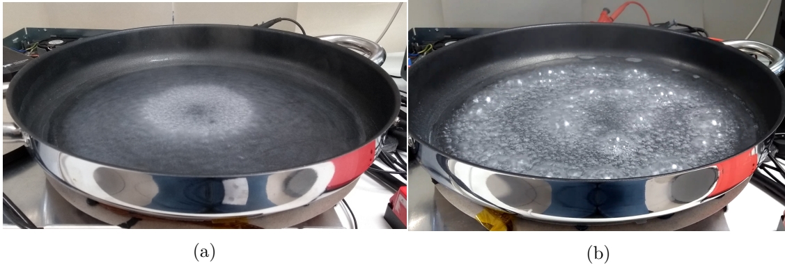
Figure 4.20: Water boiling at high power with secondary inductor (a) off and (b) on.
