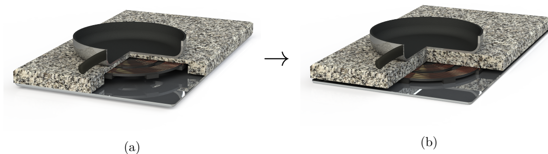
Figure 2.2: Visual representation of IuW systems: (a) commercially available, (b) proposed structure.
