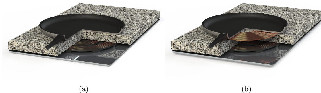
Figure 3.1: IuW implementations with (a) single inductor, (b) ICH.
