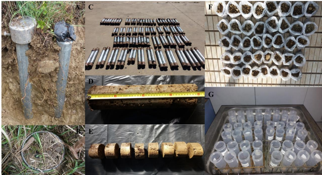
Figure 2.10. Soil sampling, preparation and analysis. A, B: Soil sampling using steel cores. C: Organizing soil samples before laboratory preparation. D: Extracting soil samples from cores. E: Sectioning references samples. F: Air drying. G: Laboratory analysis at the Pyrenean Institute of Ecology (IPE-CSIC).
