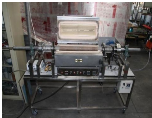
Figure 2.5 Pilot plant used for the synthesis of CNF by CDB.
