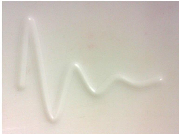
Fig. 17 a Profile of the damped function and CAD importation. b Result of the milling in a polyoxymethylene (POM) block
