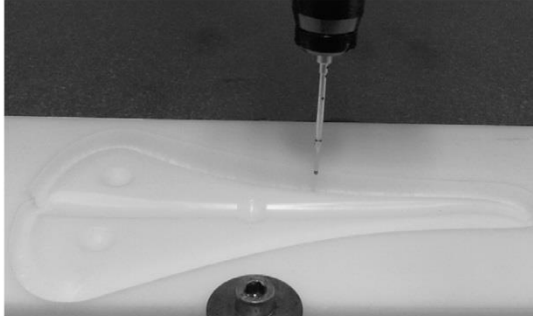
Fig. 24. Verifying the piece with a coordinate-measuring machine.
