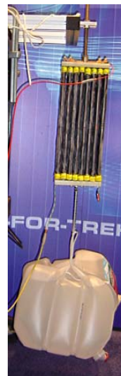
FIGURE 5: One of the groups of EMPA's EAP actuators is shown lifting two 5-gallon water containers.
