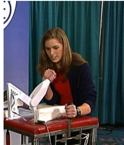
FIGURE 3: The ERI arm wrestling with the 17-year old human opponent, Panna Felsen. This arm has the size of an average human arm and it held for 26-seconds against Panna.
