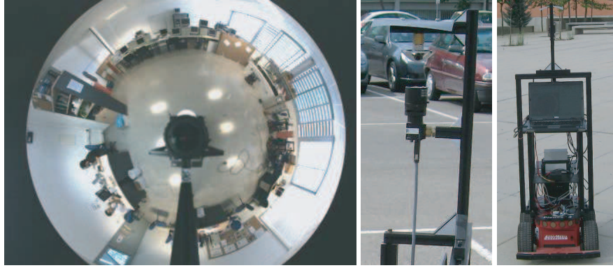
Figure 6: Example image (left), omnidirectional camera (center) and complete setup (right) used for the experiments.
