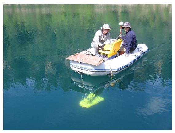
Figure 3.3: Seismic profiling during the geophysical survey in Lake El Tejo.
