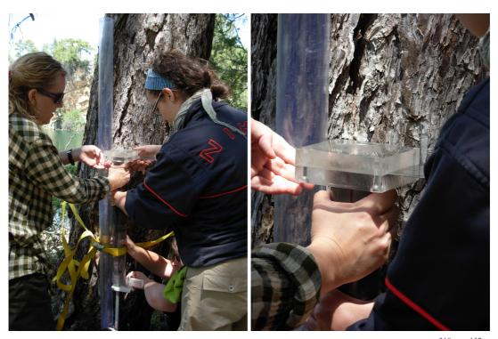
*Figure 3.10*: Field sampling of slices from the short cores recovered in La Parra for <sup>210</sup>Pb-<sup>137</sup>Cs dating.
