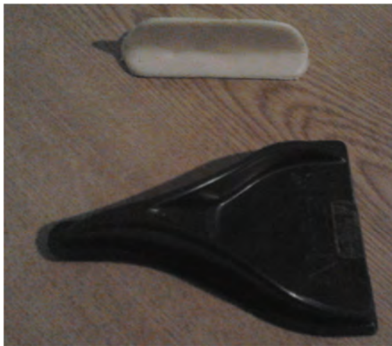
Fig 2. Rectangular shape VG (up) and Air Tab VG (down)
