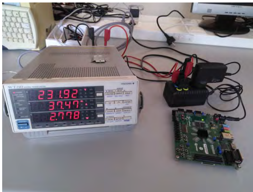
Fig. 6. Power measurement setup
