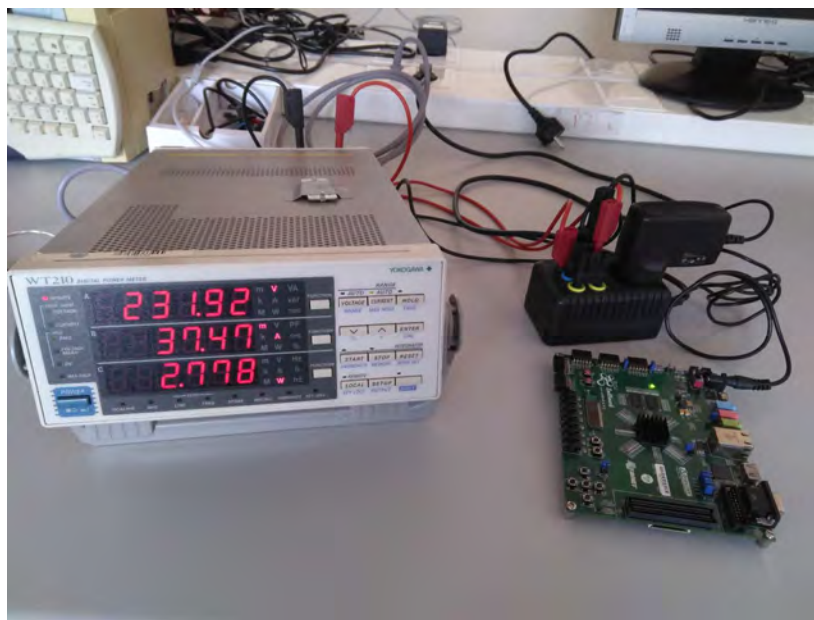
Fig. 6. Power measurement setup
