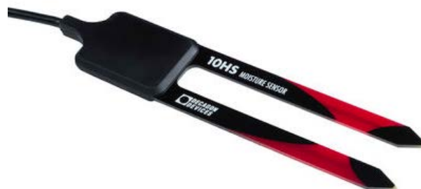
Figura 8. Decagon 10 HS soil moisture sensor
