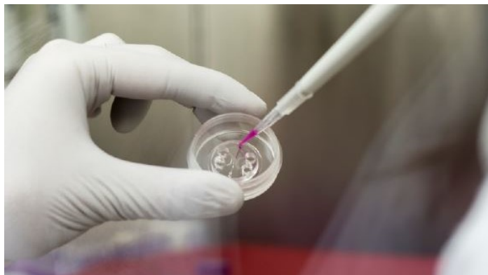
FIGURE 2.6: Pipetting the hydrogel inside the microfluidic device
