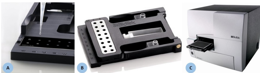
FIGURE 2.9: A: dropping DNA solutions in the microplates. B: tool filled and ready to run the measurement. C: spectrophotometer Biotek Synergy HT.
