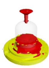
Filling Temperature (Celsius), State 14 : 22.198 seconds
