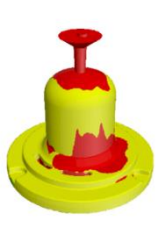
Filling Temperature (Celsius), State 20 : 31.964 seconds
