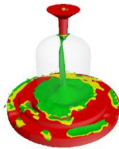
Filling Fill Rate, State 15 : 23.818 seconds
