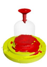
Filling Temperature (Celsius), State 13 : 20.592 seconds
