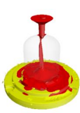
Filling Temperature (Celsius), State 12 : 18.865 seconds
