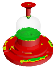
Filling Fill Rate, State 18 : 28.712 seconds
