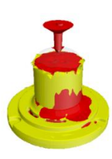
Filling Temperature (Celsius), State 19 : 31.322 seconds
