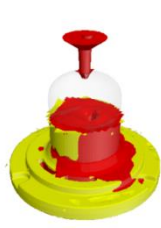
Filling Temperature (Celsius), State 16 : 25.450 seconds
