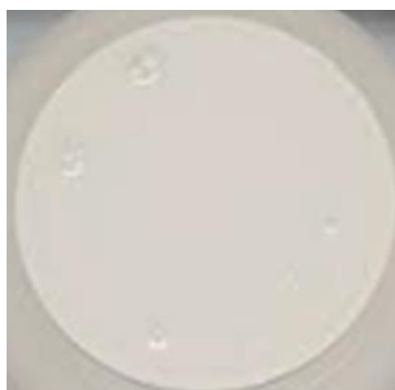
Figure A. 11. Image of NiNL-5. The formation of bubbles due the presence in excess of the surfactant led to multiple defects formation on the ceramic support.
