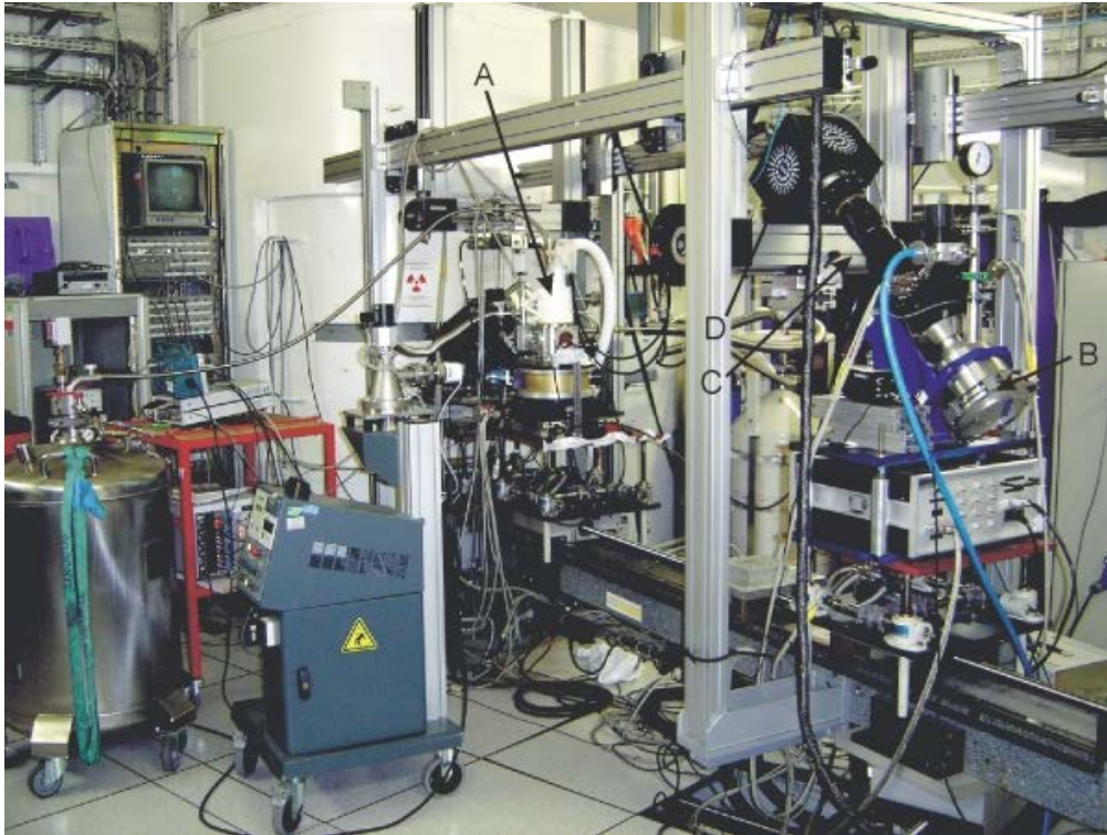
Figure 2.15. Overview of the ID24 beamline experimental hutch. A – the sample cryostat with the pulsed field coil (see Figure 2.16 for detailed view), B – fluorescent P47 phosphor screen with 100 ns for 10% afterglow and 3 \mu s for 1% afterglow, C – 25 mm diameter multichannel-plate image intensifier with 100 ns minimum gating, D – FReLoN (Fast Read Low Noise) CCD camera. Parts B, C and D of the optic/electronic system are connected by high-aperture tandem lens system.
