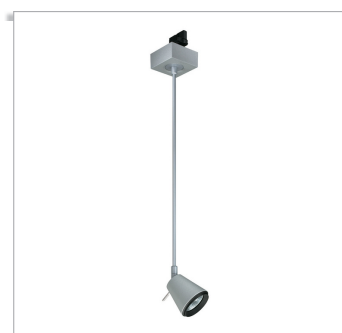
UnicOne Pendant Micro LRS/MRS541 for track mounting, with MASTERColour lamp and narrow or medium-beam optic and 600 mm extension rod (L600)
