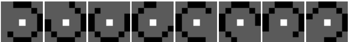
Figure 3.9: A subset of the 16 kernels used to obtain corner responses in the images. The 12 black pixels have a value of -1/12 , the gray pixels are set to 0, and the white pixel is set to 1. A very positive or a very negative response will be obtained when convolving these kernels with a corner area in an image.
