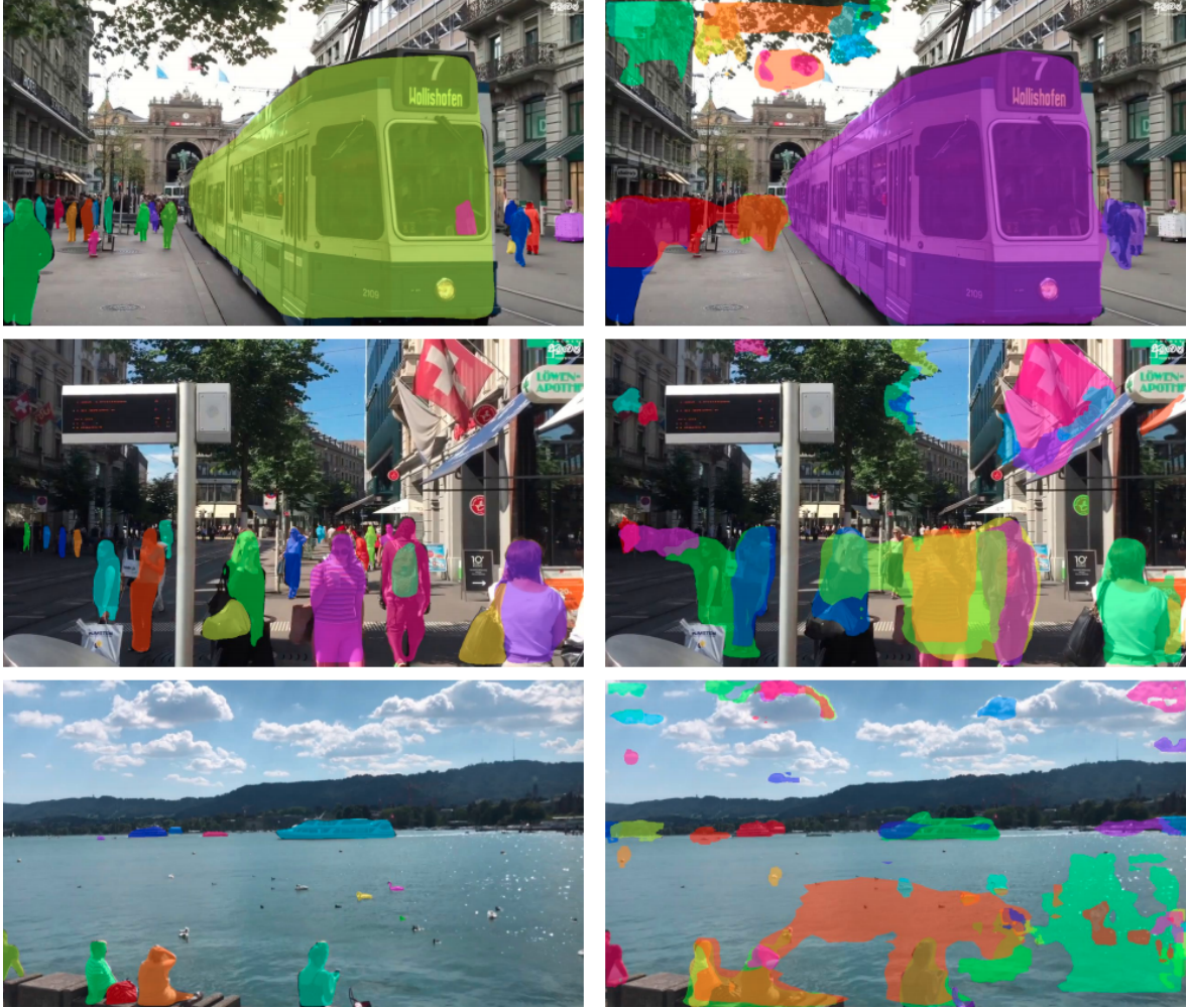
Figure 2.5: Qualitative analysis of the proposed dynamic instance detection compared to a standard semantic segmentation. Note how our algorithm trained on real-world data manages to capture the location-specific dynamic objects, such as trees or flags.
