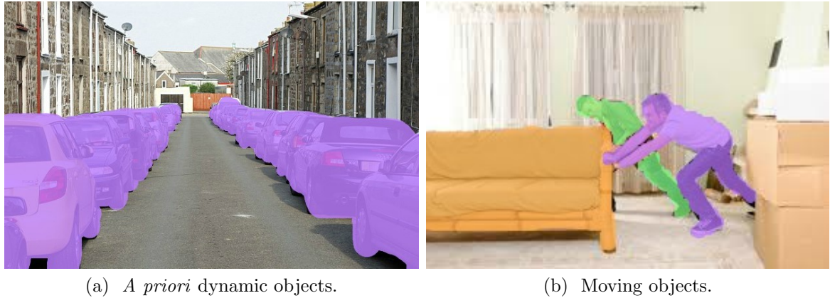
Figure 1.7: Whereas geometry-based approaches are used to detect scene movement, semantic information can be utilized to detect a priori dynamic classes.
