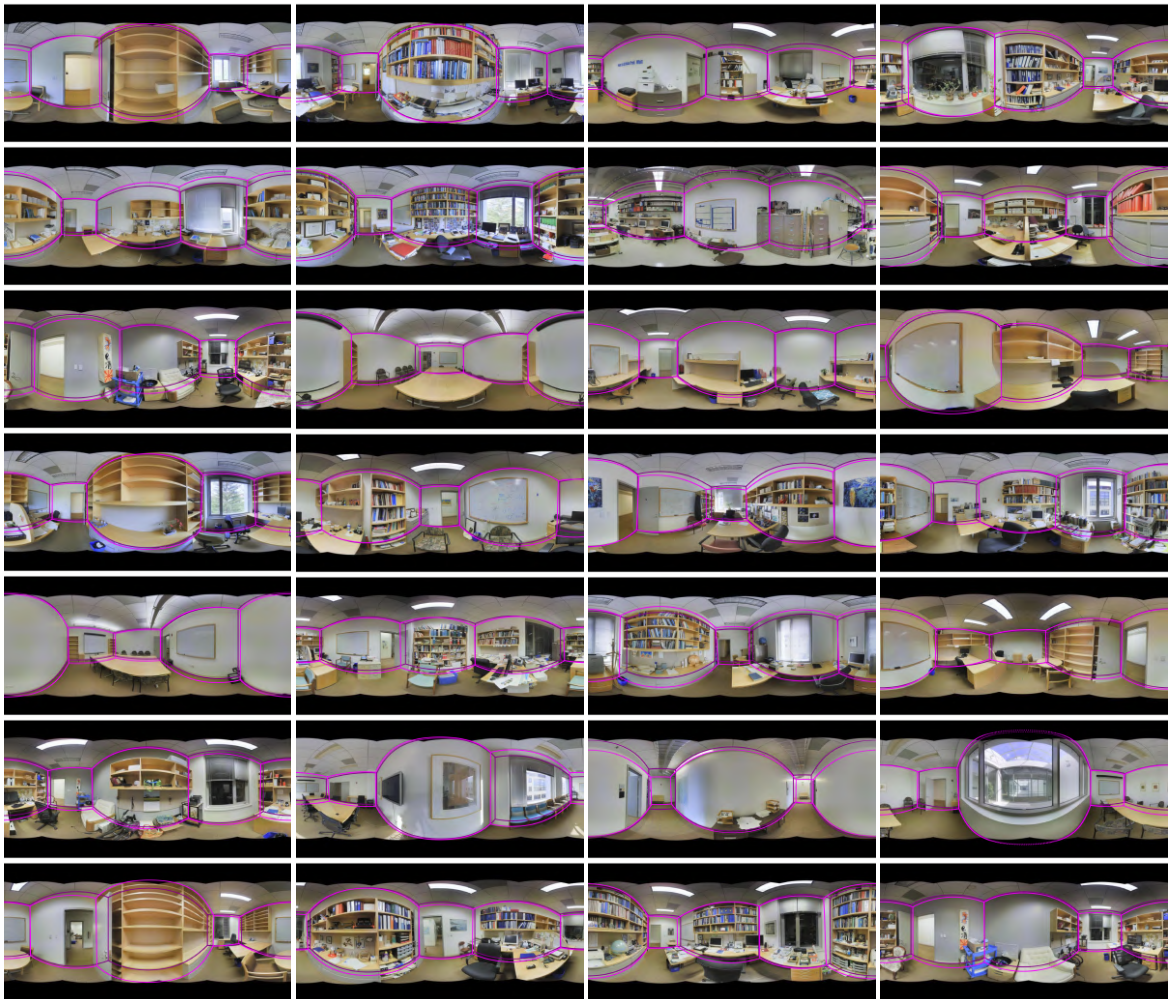
Fig. 5.13 Layout predictions (light magenta) and ground truth (dark magenta) on the Stanford 2D-3D annotation dataset (Armeni et al., 2017). Best viewed in color.
