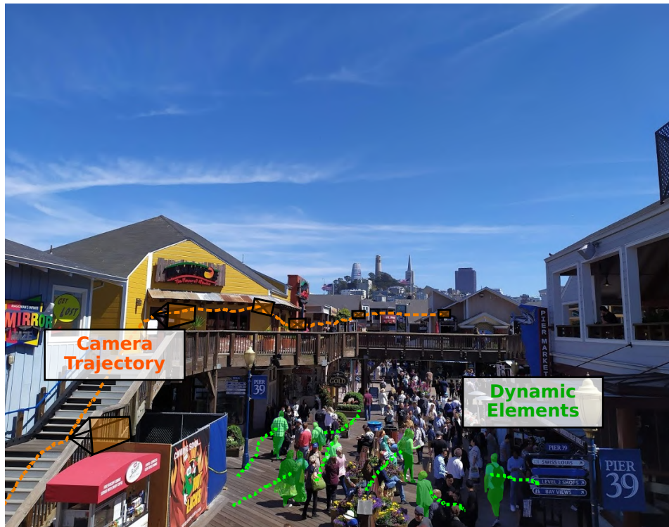
Fig. 1.6 This image shows an example of how dynamic objects are detected over time and taken into account when tracking the camera position. At the same time, the map could be built, not considering the dynamic objects because they should not be part of it.
