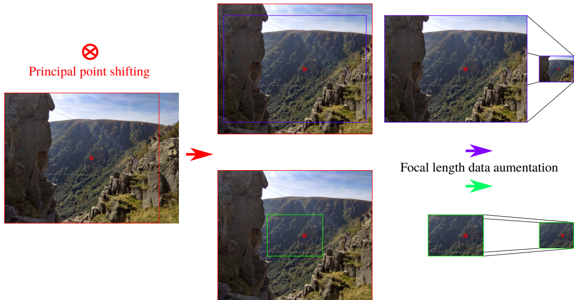
Fig. A.3 Overview of the steps for camera data augmentation.
