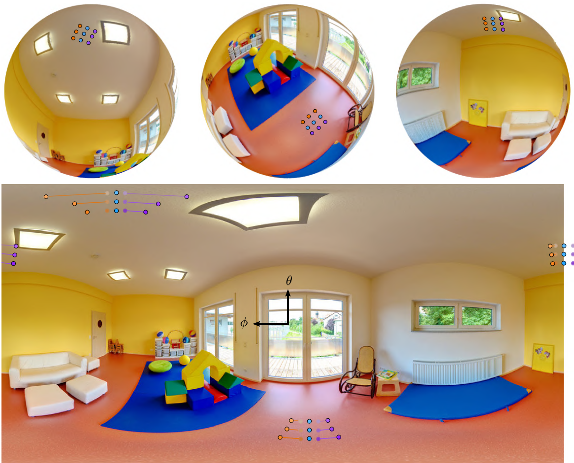
Fig. 5.6 EquiConvs on spherical images. We show three kernel positions to highlight the differences between the offsets. As we approach to the poles (larger \theta angles) the deformation of the kernel on the equirectangular image is bigger, in order to reproduce a regular kernel on the sphere surface. Additionally, with EquiConvs, we do not use padding when the kernel is on the border of the image since offsets take the points to their correct position on the other side of the 360^\circ image.
