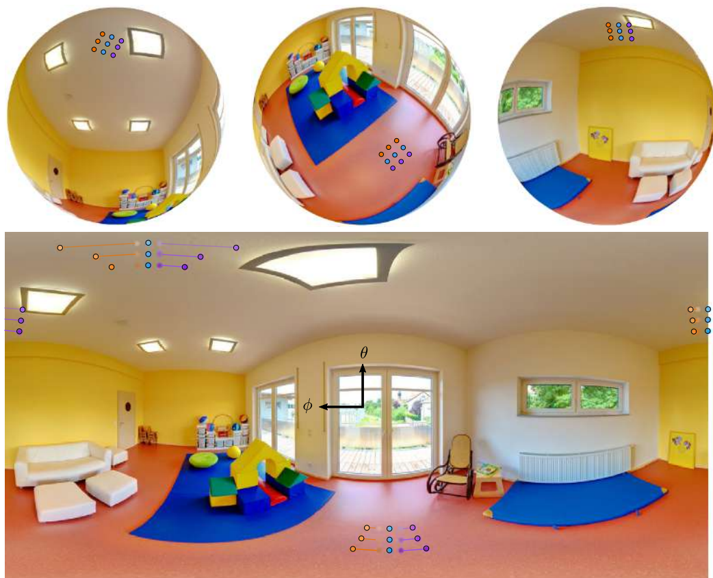
Fig. 2.20 EquiConvs on spherical images. We show three kernel positions to highlight the differences between the offsets. As we approach to the poles (larger \theta angles) the deformation of the kernel on the equirectangular image is bigger, in order to reproduce a regular kernel on the sphere surface. Additionally, with EquiConvs, we do not use padding when the kernel is on the border of the image since offsets take the points to their correct position on the other side of the 360° image.
