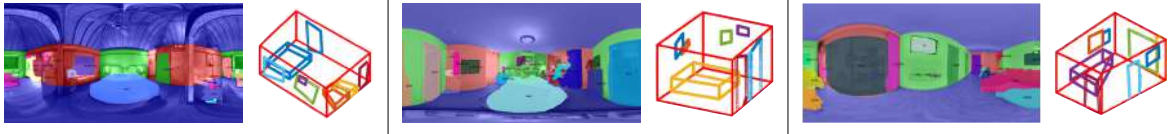
Fig. 3.3 Examples of 3D models obtained from instance objects masks and room layout knowledge [41].
