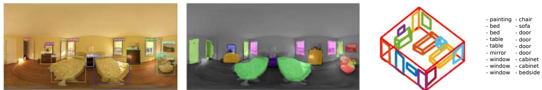
(b) Scene level: localization and segmentation of objects and their distribution in the 3D scene.
