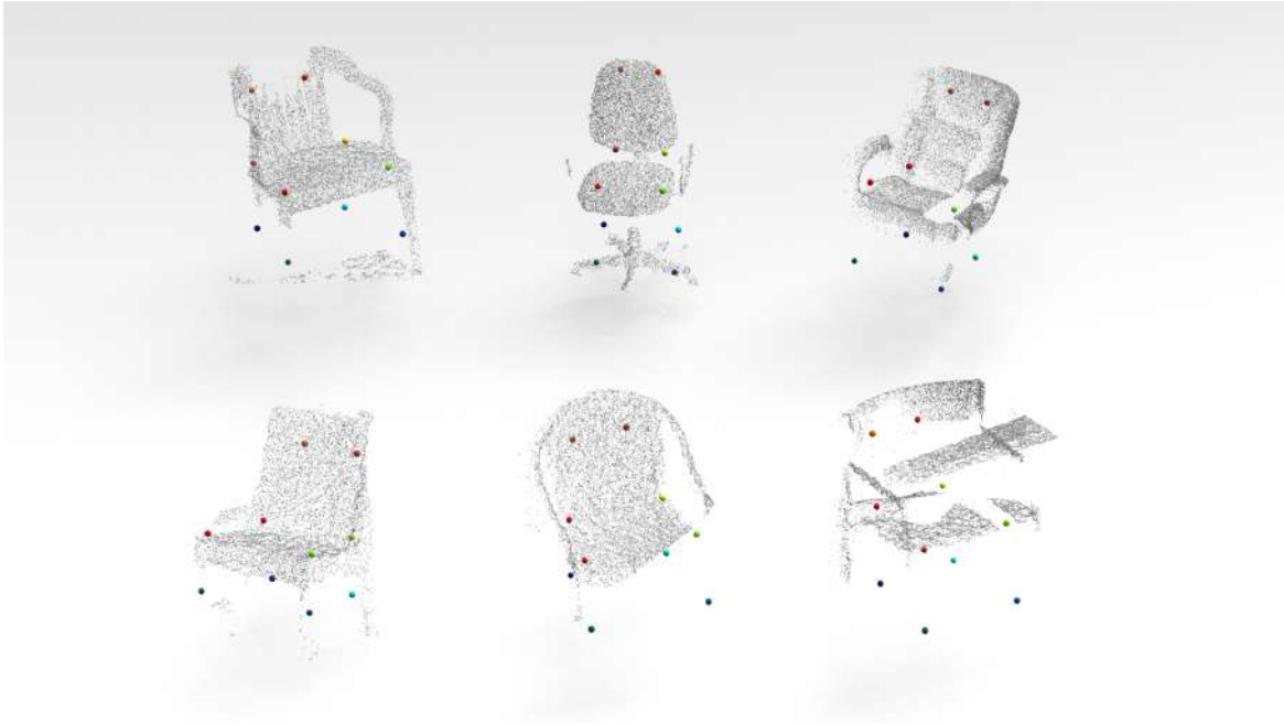
Fig. 4.8 Results in real chairs from SUNRGBD dataset [131] training with CAD chairs from ModelNet10 dataset [157].
