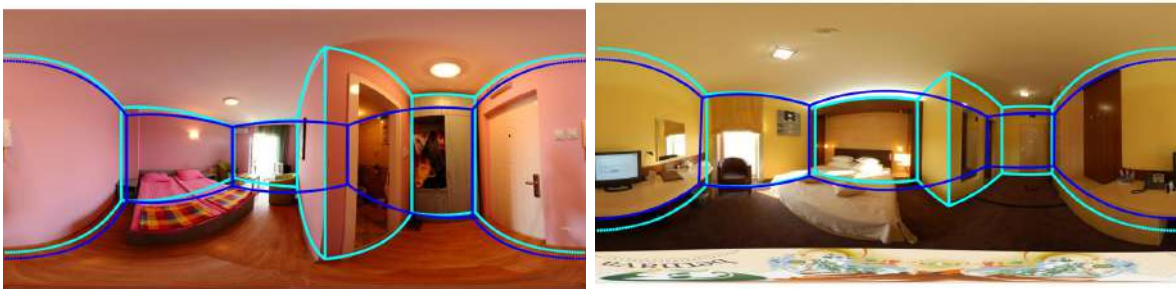
Fig. 2.10 Comparison with PanoContext [172] in complex geometries. Our method (cyan) is able to find 6 walls whereas [172] (dark blue) always finds just 4 walls.
