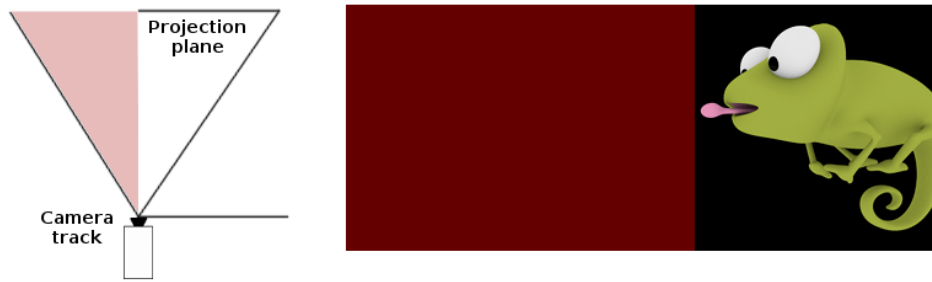
Figure 4.5: The camera is characterised by a wider field of view. The unnecessary region of the image is dismissed in the image on the right.
