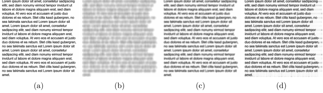
Figure 5.2: a) Original text image. 75 iterative zoom-in&zoom-out scaling, factor \sqrt{2} b) by bilinear algorithm, c) by bicubic algorithm, d) by Fast DCT algorithm.
