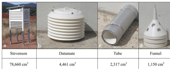
Fig. 2. The Stevenson, Datamate ACS-5050, tube and funnel radiation shields. Total volume is expressed in cubic centimeters (cm 3 ).
