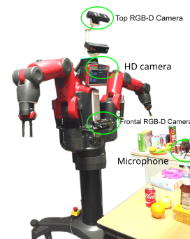
Fig. 4: Baxter robot setup used to acquire the dataset. The three cameras and the microphone locations are highlighted.
