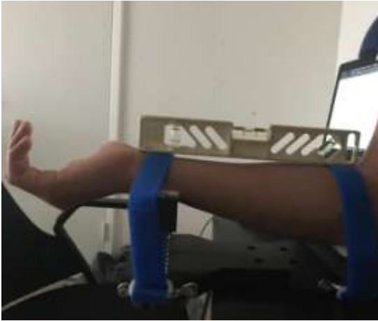
Figure 18: The arm fixture demonstrating that it can level a forearm
