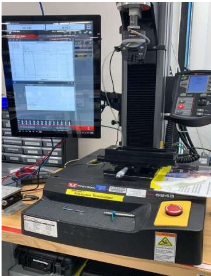
Figure 14: Instron configuration with designed Fixture.
