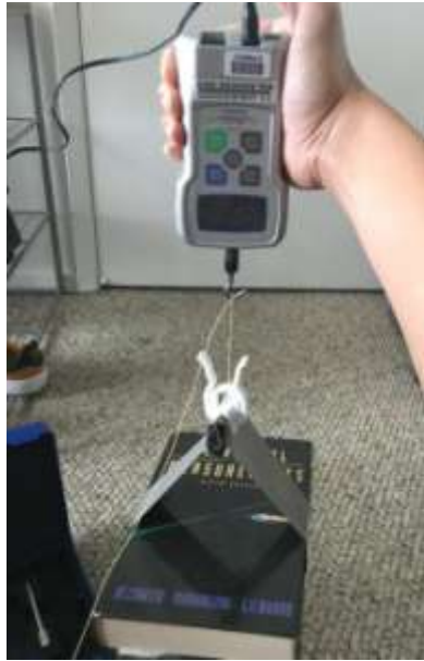
Figure 19: Prototype clamp demonstrating that it can grip 2.74 lbs
