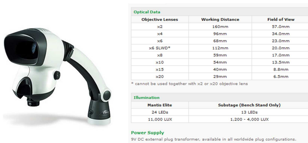
Figure 5.5: Technical specifications of the Mantis Elite ® magnifying glass.
