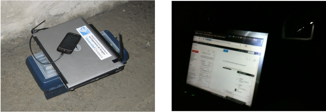
Figure A.11: Laptop used as gateway and laptop used as mobile node along the tunnel.
