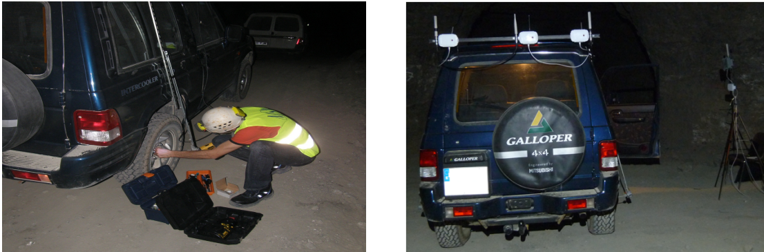
Figure A.5: Mapping wireless coverage - Santa Marta mine
