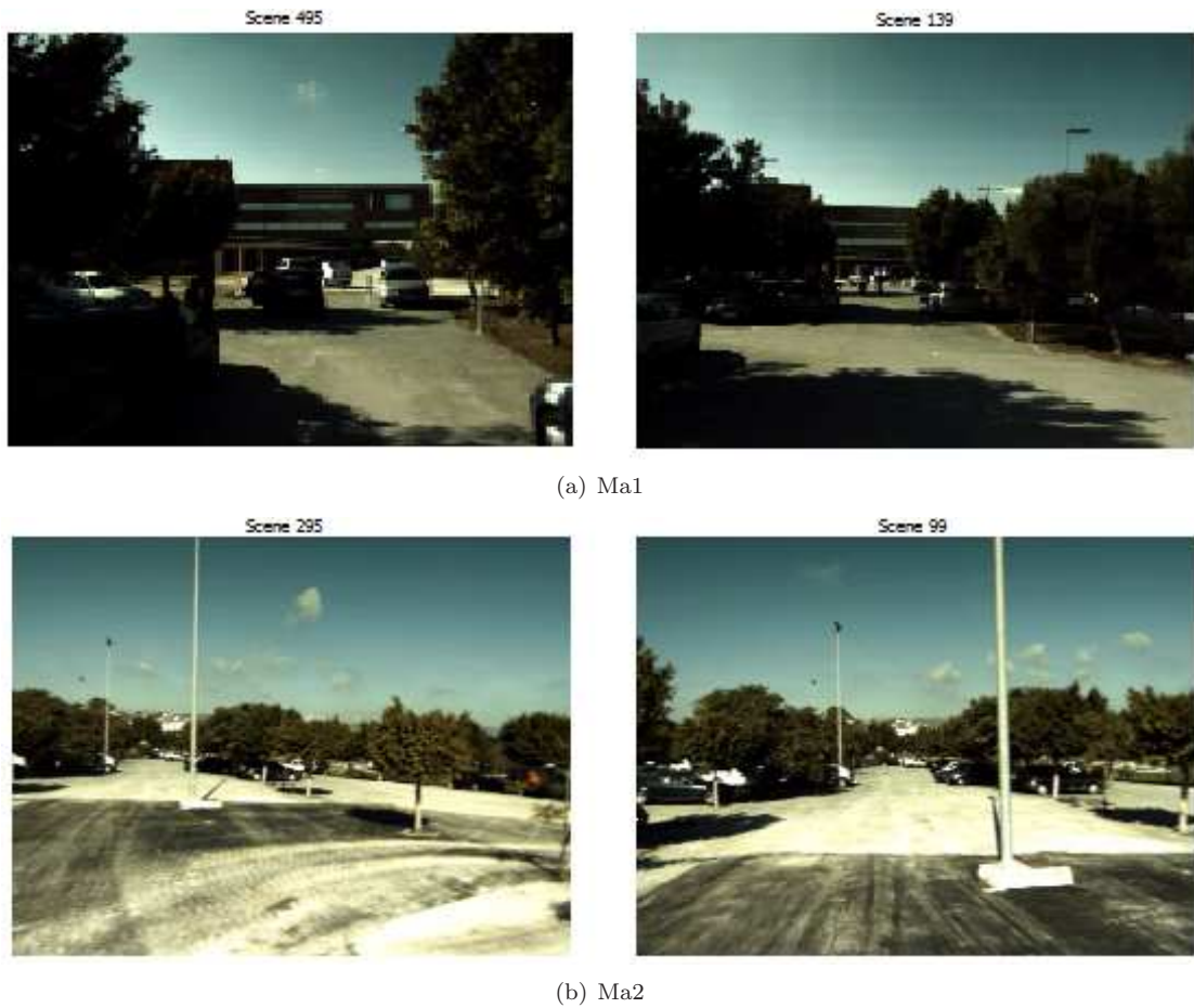
Figure 3.26: Cases marked in Figure 3.25(b) and Figure 3.25(d) from Malaga6L dataset. Case (a) Ma1 is a loop found by our BoW + CRF-Matching approach. Case (b) Ma2 is a loop found by FAB-MAP 2.0 (default) + GC. Places are correctly recognized although the position of the cameras are some meters apart. Both cases are considered as true positives.
