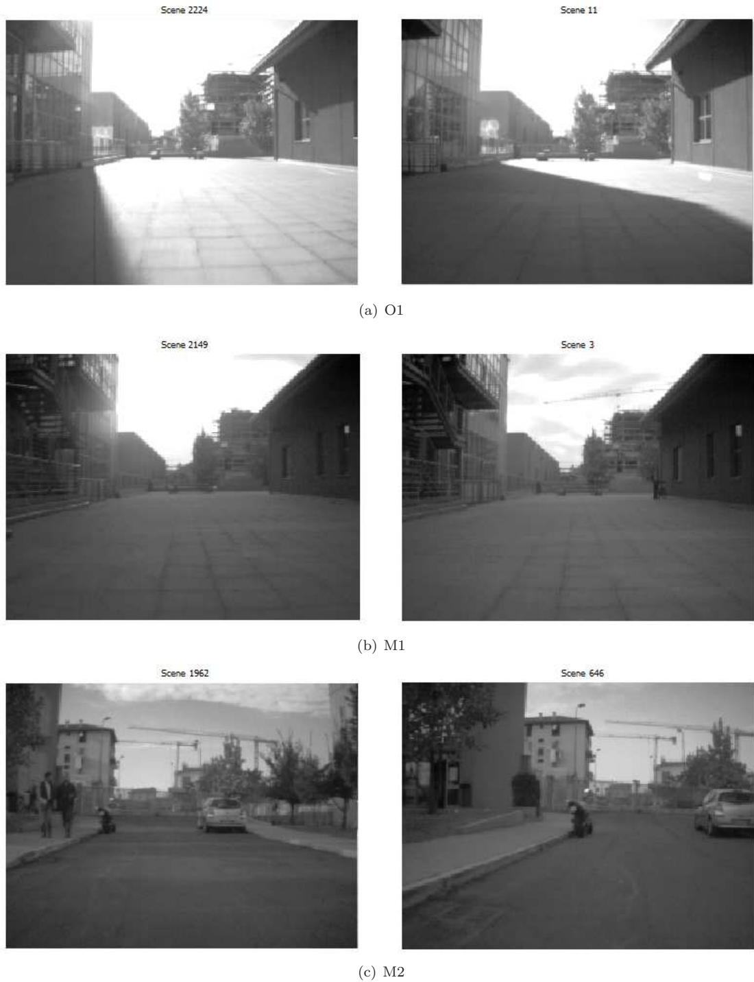
Figure 3.24: False negatives in the Bovisa04 and Bovisa06 datasets that our method can successfully detect but FAB-MAP 2.0 misses. FAB-MAP 2.0 sets query image of case (a) as new place with a probability of 0.99947; of (b) with 0.99997 and 0.99902 with the default and modified set of parameters respectively, and of (c) with 1.0 and 0.9993. These scenes correspond to the biggest loops in the trajectories.
