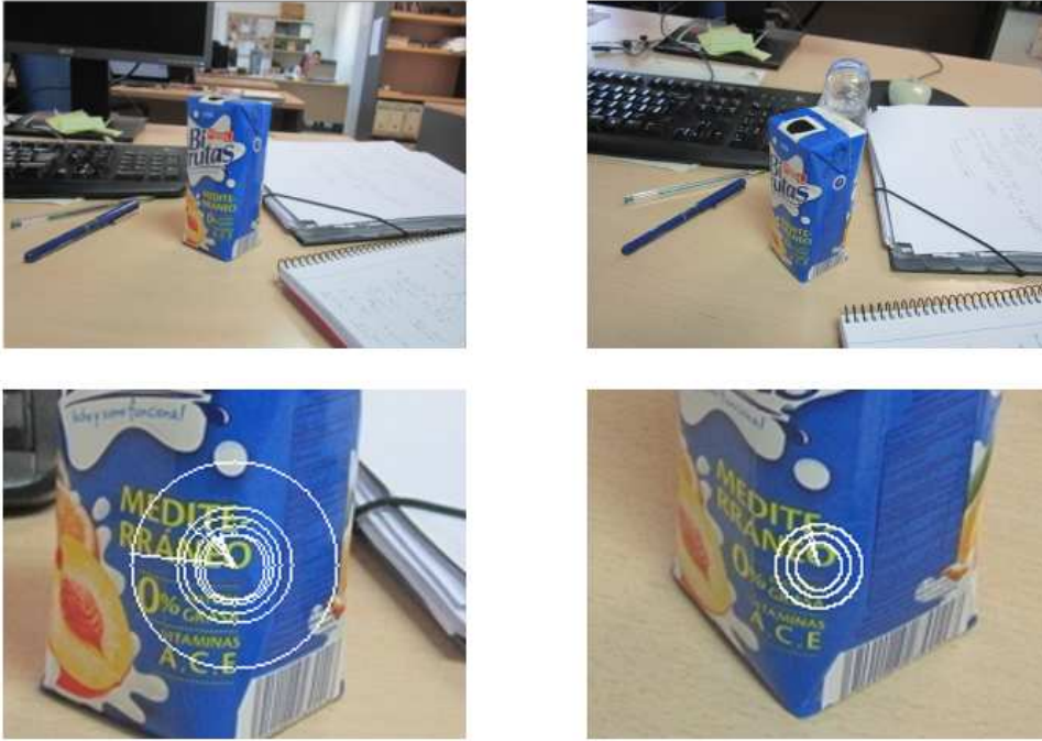
Figure 5.8: The description of a 3D point is obtained from several ORB descriptors when creating the model. Top row: two training images of a juice box. Bottom row: zoom in showing the ORB features obtained at several scales from the same 3D point seen in the two training images. All these descriptors are converted into visual words. Descriptors that result in the same word are merged to disregard redundant information.
