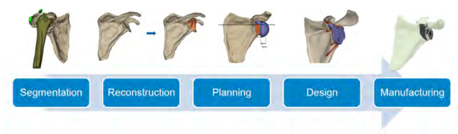
Figure 2.8: The different steps in the design and manufacturing of the Glenius system (courtesy of Materialise NV).
