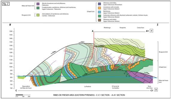
Figure 2. Cross-section of the El Baell unit.
