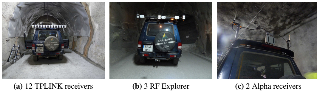
Figure A.3: All-terrain vehicle: RF sensors layouts.
