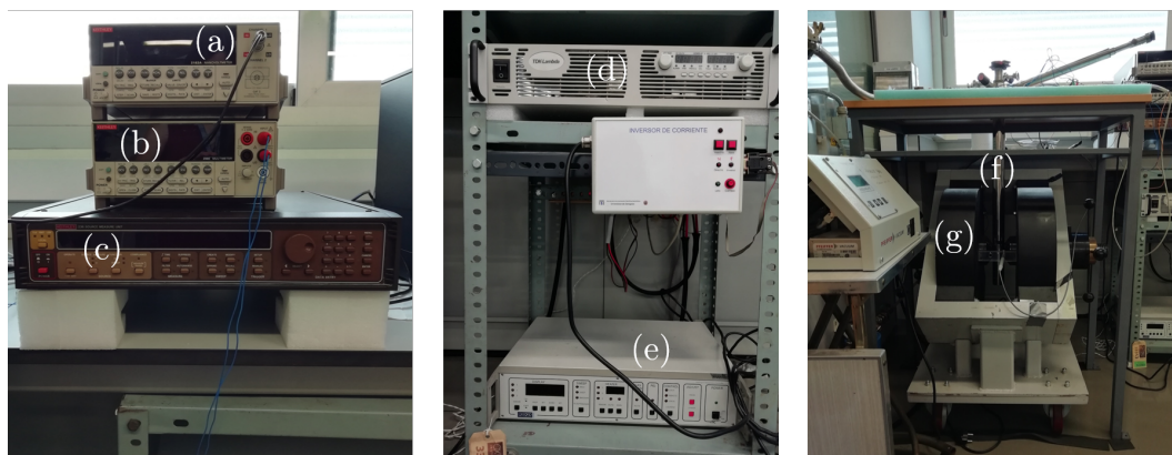
Figure 2.11 Transport measurement system components. (a) Keithley 2182a nanovoltmeter. (b) Keithley 2000 multimeter. (c) Keithley 236 SMU. (d) Electromagnet TDK Lambda power source. (e) Temperature controller. (f) Cryostat. (g) Electromagnet.
