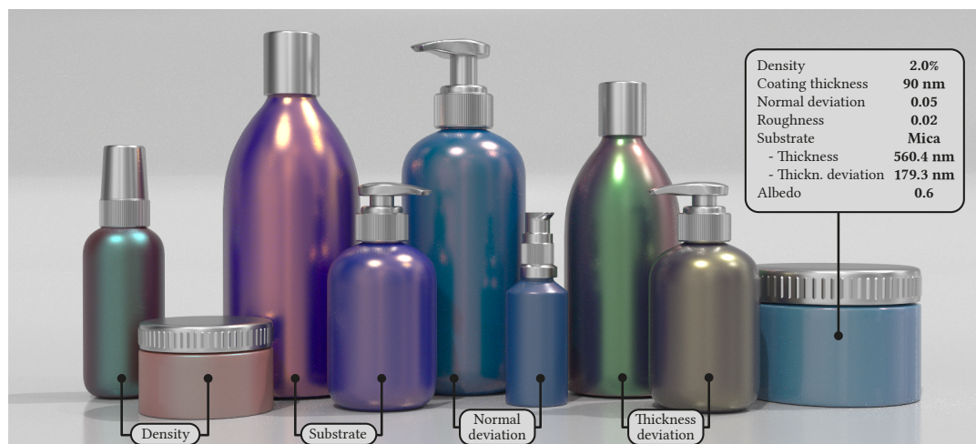
Figure 3.1: Synthetic objects rendered using our pearlescent material model, showing how changing a single parameter in each pair of bottles (as indicated by the brackets) leads to large, difficult-to-predict changes in appearance. From left to right, the changed parameters are: a) platelet density variation; b) substrate composition; c) deviation of the platelet normal distribution; d) deviation of the substrate thickness. The rightmost jar shows the values of our model parameters for its particular material. Please refer to Table A3 for a complete description of all the materials.
