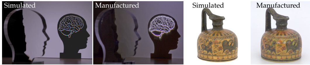
Figure 1.3: Examples of predictive rendering. Left: A glass object designed to project a certain refraction pattern when illuminated from behind. The surface of the object was computationally optimized by simulating the light transport inside the object until its refraction converged to the desired pattern. Right: A 3D printed object designed to display a well-defined and high contrast texture pattern on its surface. The distribution of pigments in the inner layers of the object was optimized to reduce color bleeding and color washing, caused by light scattering by the highly transparent thermoplastic resins. Left images from: [189]. Right images from: [210].
