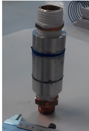
(b) Half mounted canister assembly. The central disposition of the packed bed allows for a symmetric assembly. The sealant forms a gasket that glues the surfaces together with the mesh.
