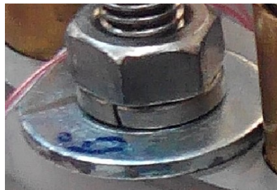
Figure 4.11: Split-lock washer used to avoid loosening of the AMR block. This special washer is placed between the nut and a normal flat washer. This last washer has a bigger diameter and has a smooth surface, protecting thus the surface of the home designed pressure leveling washer while helping in the pressure distribution.
