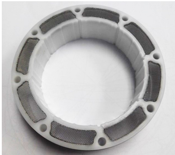
Figure 4.17: An AMR section with its meshes glued in place.
