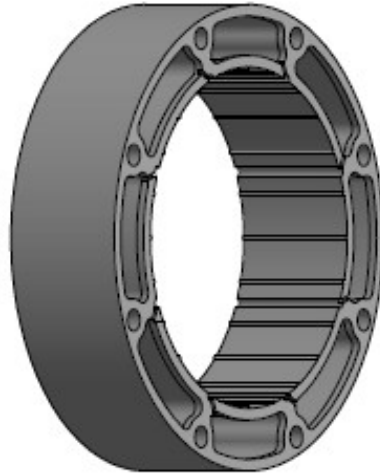
Figure 4.6: Perspective of the design of the AMR sections . The lobed design contributes to a smoother transition between regenerators while avoiding stress concentration points. The core of the magnet is inserted in the central hole and the regenerator makes contact only with the small vertical protruding ribs shown, creating a small air chamber acting as thermal insulation.
