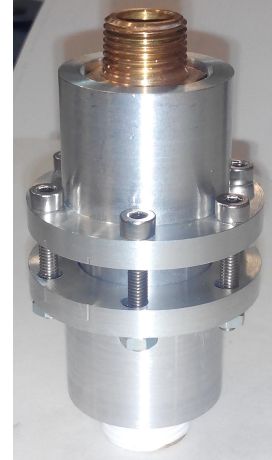
(c) Completely mounted canister assembly. The canister cylinders are pressed together to form a watertight assembly. Teflon tape is applied to the thread to avoid leaks.
