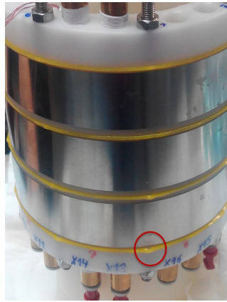
(a) Outwards extrusion of the gasket in one of the tests, marked in a maroon circle.
