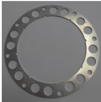
Figure 4.8: Home designed laser cut pressure washer meant to distribute the closing pressure of the nuts and threaded rods more homogeneously. This washer can be seen once assembled in figure 4.10b.
