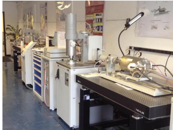
Figure 3.1: Thermo-physical measurements Lab at CERN. Right side: horizontal dilatometer (DIL 402E). Next to the left: vertical Laser Flash machine (LFA427).
