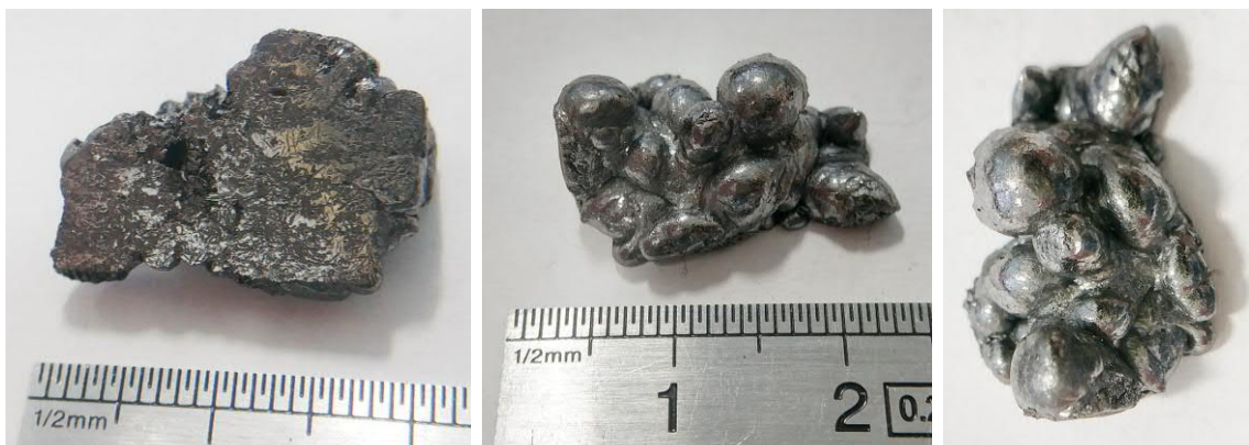
Figure 6.29: Cr-C LP spill material from CG-1100B0 plate. One surface was polished to reveal its internal structure, which shows visible grown graphite flakes (left).
