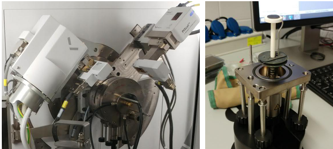
Figure 3.14: (Left) X-ray diffractometer with furnace chamber. (Right) sample holder for the high temperature XRD test. Sample shown on top of it is about \text{Ø}13 \text{ mm} .
