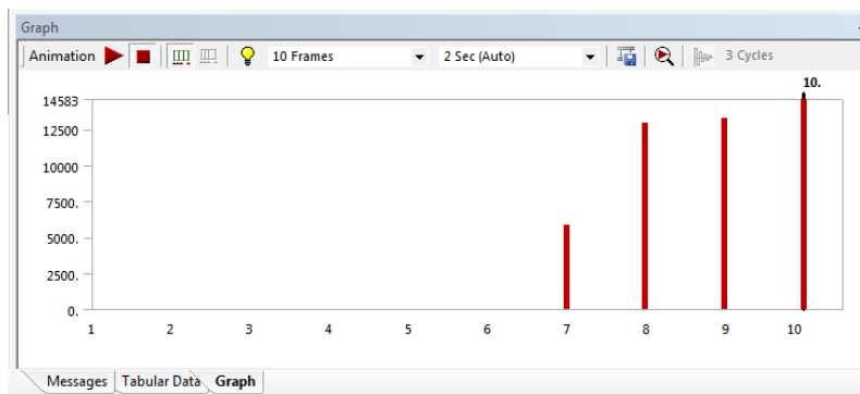
Figure E.9: Plot of the frequencies of the first 10 modes of an IP free-standing specimen. The first 6 modes with F \approx 0 Hz are the degrees of freedom.
