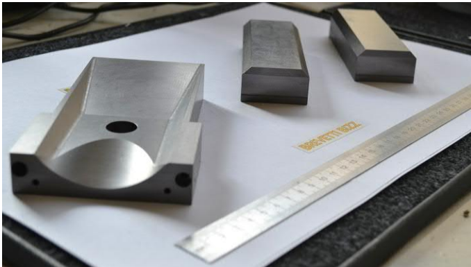
(a) MG-6530Aa machined blocks for full-size collimator test. External dimensions of the parts shown are 150 \times 100 \times 25 \text{ mm} or 125 \times 45 \times 25 \text{ mm}
