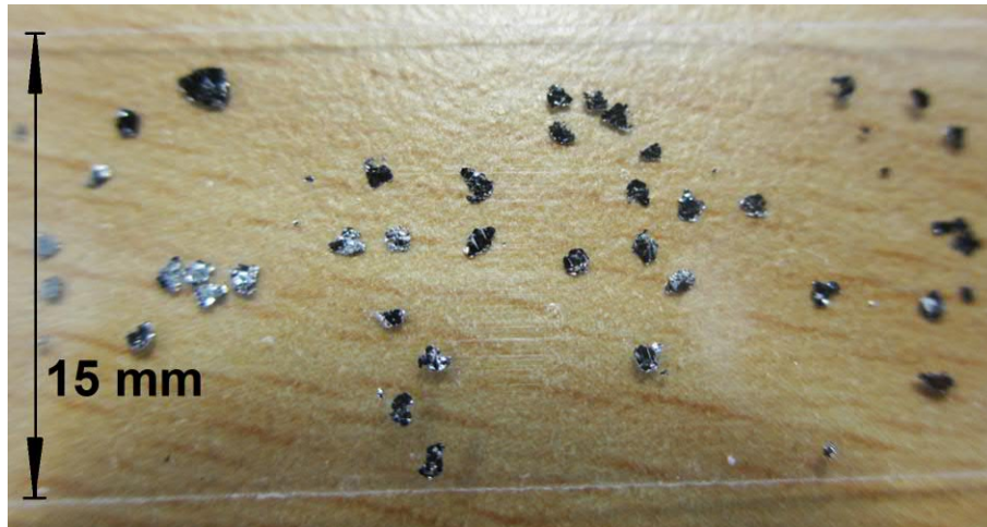
Figure 4.12: Asbury 3763 graphite powder on adhesive tape.
