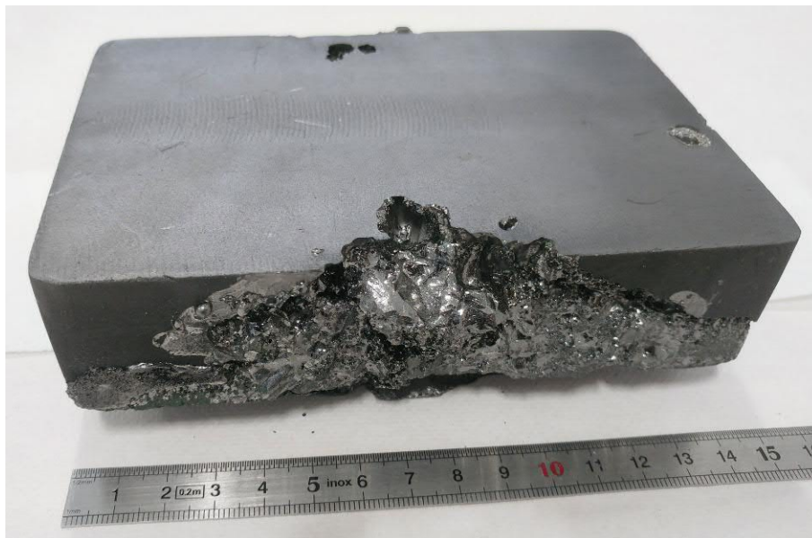
Figure 6.25: Upper graphite punch used to sinter CG-1240X plate, showing extensive dissolution by the Cr-C liquid phase.
