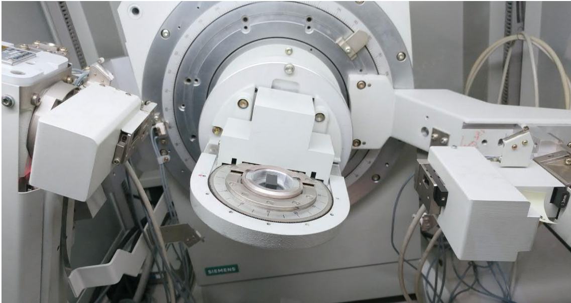
Figure 3.13: Siemens D5000 X-ray diffractometer, testing a graphite sample ( \sim 10 \times 10 \times 25 mm).
