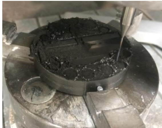
Figure 4.35: Milling specimens from a sintered plate
