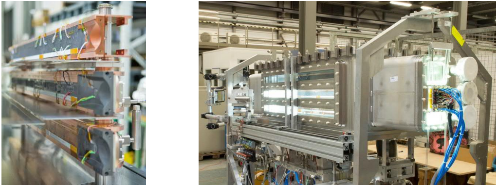
Figure 1.29: The three collimator jaws and the vacuum tank of the HRMT23 experiment. The top jaw is made of a single piece of CFC AC150K and GLIDCOP ® Al-15 taperings, the middle one is made of MoGr blocks and taperings and the bottom one has copper-diamond blocks and MoGr taperings.
