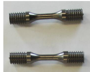
(b) Example of MG-6541Aa specimens for dynamic tests machined by Brevetti Bizz. Length is 30 \text{ mm} and threads are M6
