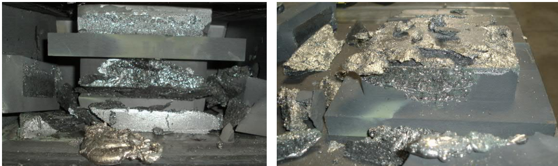
Figure 5.83: Sintering failure of plate CG-1240X. Plate surface is 150×100 mm.
