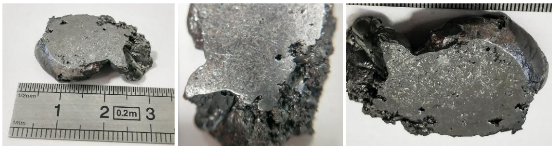
Figure 6.28: Cr-C LP spill material from CG-1100A0 plate. One surface was polished to reveal its internal structure.
