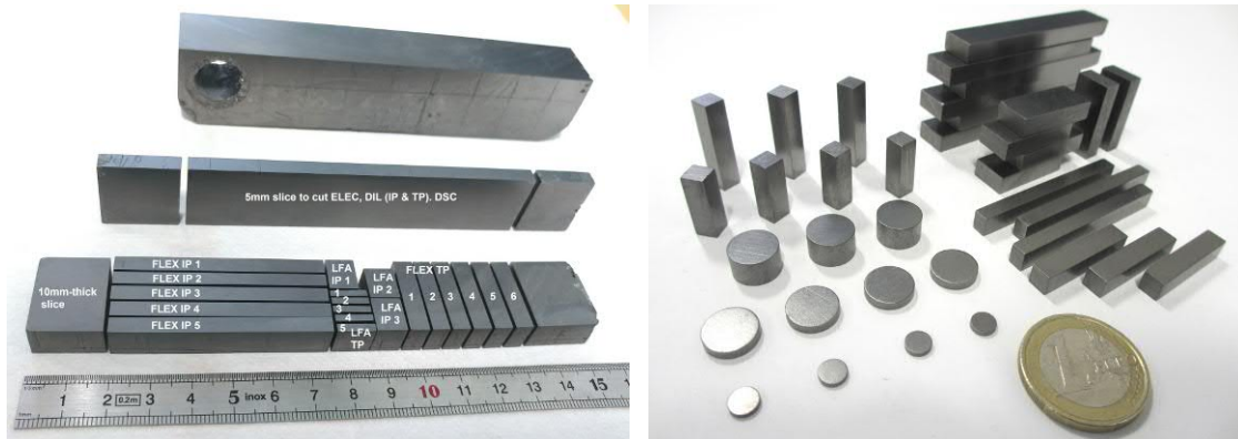
Figure 4.39: (Left) Samples extracted with the diamond wire saw. (Right) Samples milled by the supplier.
