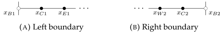
FIGURE 2.6: Boundary zones in a one-dimensional domain. The circles at edges correspond to known values with Dirichlet BC.
