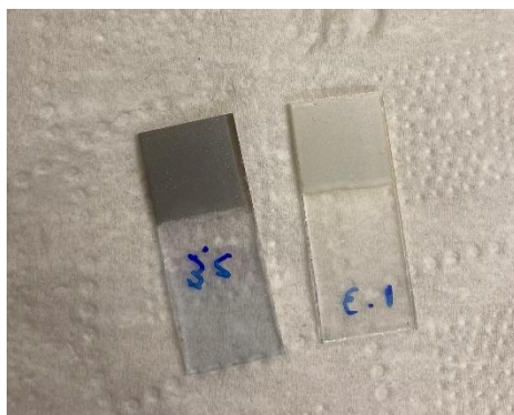
Figure 14. Anodes \text{TiO}_2/\text{rGO} (left) and \text{TiO}_2/\text{GO} (right).
