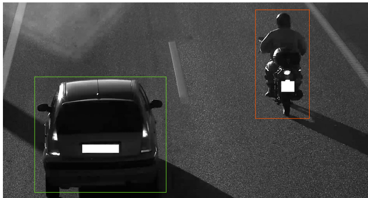
Figure 3.9: Graphic interpretation of the output of a DNN used for detection and classification tasks. The image has been provided by Lector Vision S.L.
