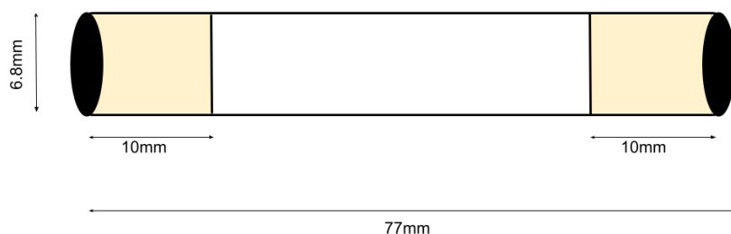
Figure B.1: Measurements of an enamelled tubular ceramic membrane.
