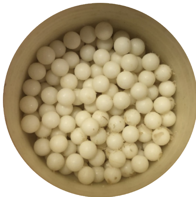
Figure A3. THEDES mechanosynthesis. Photos of the reactor at the end of the reaction of an unsuccessful reaction, benzocaine:thymol (1:1).
