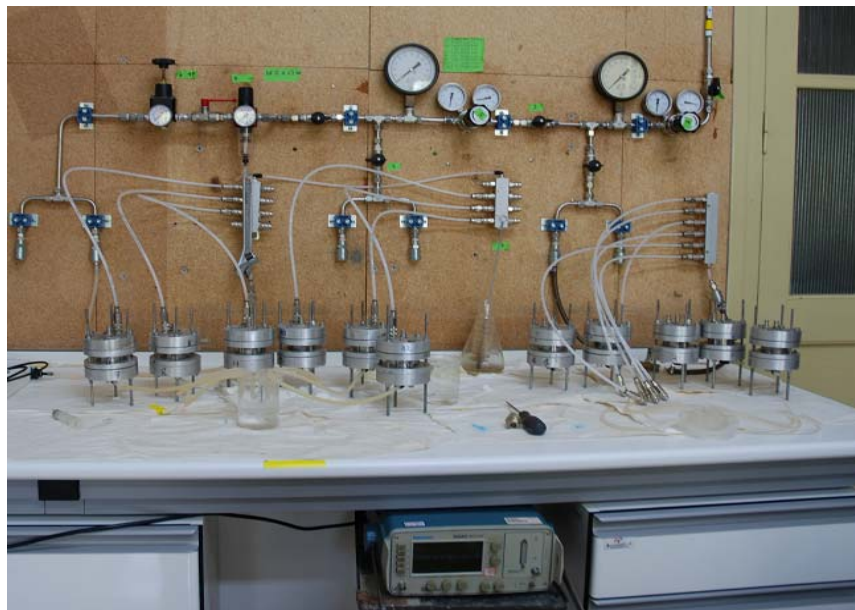
Figure 5. Set of TDR-cell to measure the water retention curve
