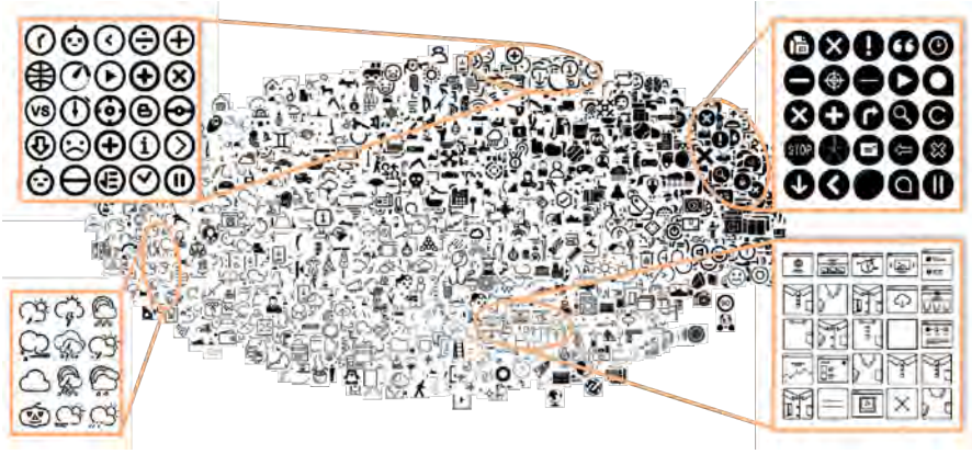
Figure 4.7: Visualization created using the t-SNE algorithm. It reduces the dimensionality of the feature vectors that our model learns to a two-dimensional Cartesian space. Note how icons with similar appearance are grouped in the same regions.
