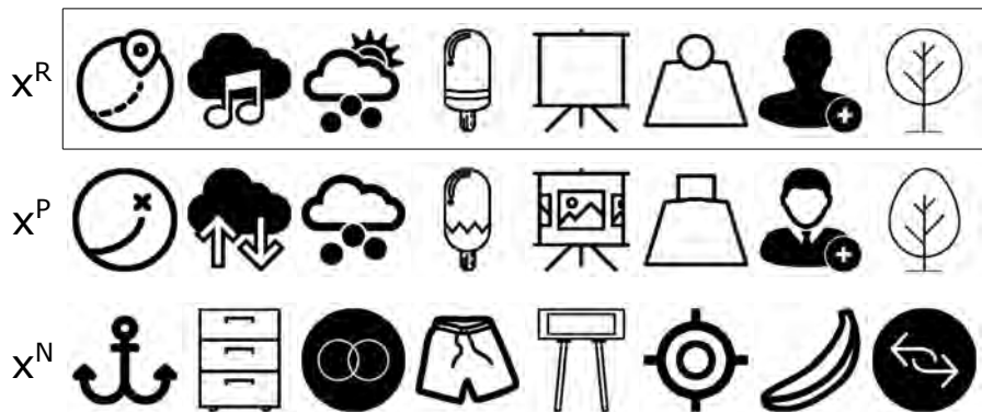
Figure 4.5: Examples of the triplets sampled during training. The variables x^R , x^P and x^N refers to the reference, positive and negative icon respectively. The positive icon and the reference are selected from the same class and they have the larger Euclidean distance among the icons inside that class. The negative icon has the shorter Euclidean distance to the reference among the icons within a different randomly selected class.
