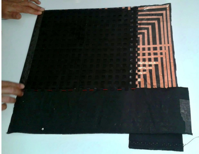
Figure 3. Developed force-sensitive resistor sensor mat.
