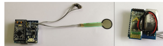
FIGURE 5: Elements of the sensing system mounted: front of the prototype with the Arduino Pro Mini, battery charger, and FSR (a) and back of the prototype with the Bluetooth module and battery (b).
