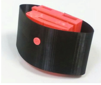
FIGURE 8: Prototype designed with all the circuitry embedded inside.
