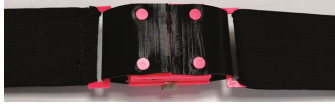
FIGURE 9: Back of the casing showing the fixation of the flexible part to the solid part. The belt is attached to both sides of the flexible part by two rings.
