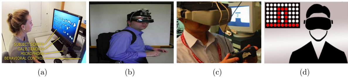
Figure 1.5: Simulated Prosthetic Vision (SPV) setups. (a) The stimulus is displayed in a computer screen in front of the subject [37]. (b) Subjects carry a PC video camera placed in a modified adjustable head strap in a midline position above the eyes. The laptop is placed in a specially designed computer backpack, making the system completely portable [38]. (c) Subjects view pixelized imagery in a head-mounted display [39] or (d) through a virtual patient [40].
