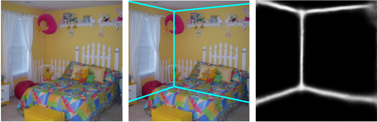
Figure 2.3: Using [119] we detect the main structure of the room extracting the structural informative edges (SIE) (right) which are those formed by the intersection of walls, ceiling and floor of the room (middle).
