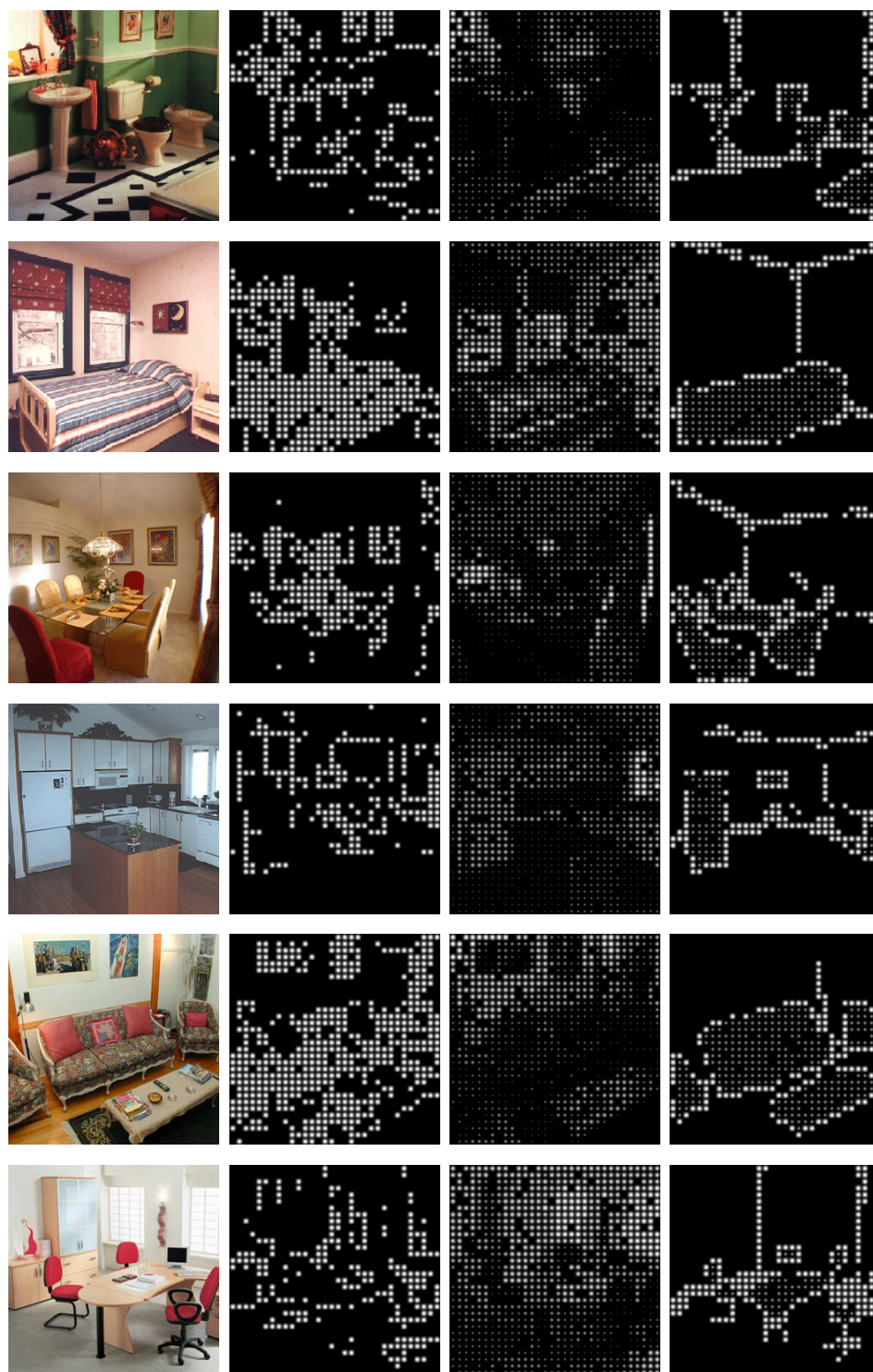
Figure 2.7: Six examples of indoor environments represented with 1024 phosphenes (rows: bathroom, bedroom, dining room, kitchen, living room and office, respectively). Each column shows: a) input images, b) images processed using the Edge method, c) images processed using the Direct method and d) images processed by our SIE-OMS method, respectively.
