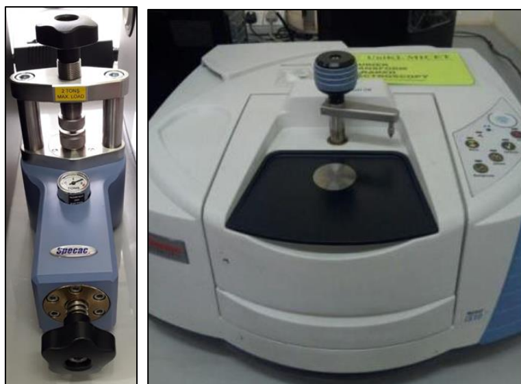
Figure 3.7 (A) Compression machine (B) Fourier Transform Infrared Spectrometer
