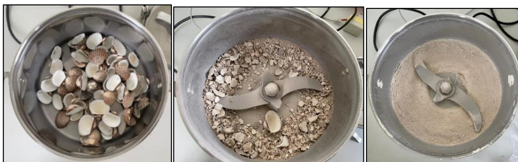
Figure 3.4 (A) The cockleshell before grinding. (B) The obtained cockleshell granule. (C) The obtained cockle shell powder
