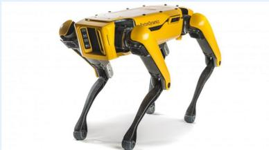
Figura 2.5: Robot Spot de Boston Dynamics [24]
