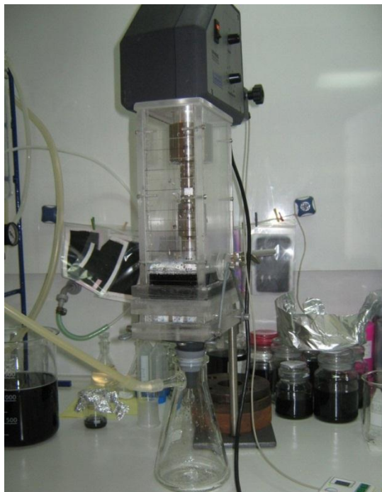
Figure 22 Tip sonication and ultrafiltration configuration. Rectangular vessel contains CNTs solution which by pressure difference is driven through membrane pores
