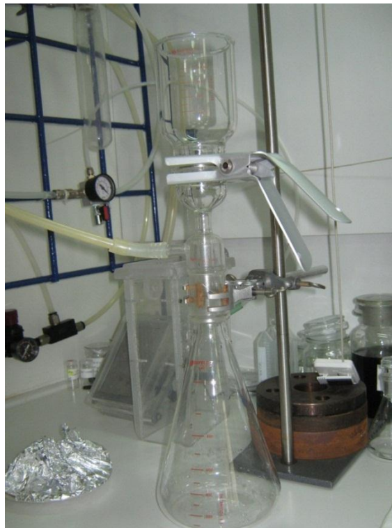
Figure 18 Ultrafiltration unit in laboratory (pressure supply, vessel, and membrane)
