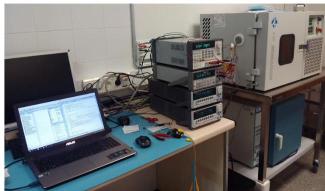
Figure 2.12. Measurement setup for the complete characterization of the LDO regulator: a) Block diagram of static (grey), transient load regulation (green) and transient line regulation (blue); and b) Experimental setup.
