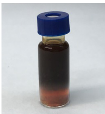
Figure S1 . Example of two-phase distribution after the co-pyrolysis of GSs and PS using a initial GSs-to-PS ratio of 80:20 (wt%/wt%). Top layer: Organic phase; down layer: Aqueous phase.
