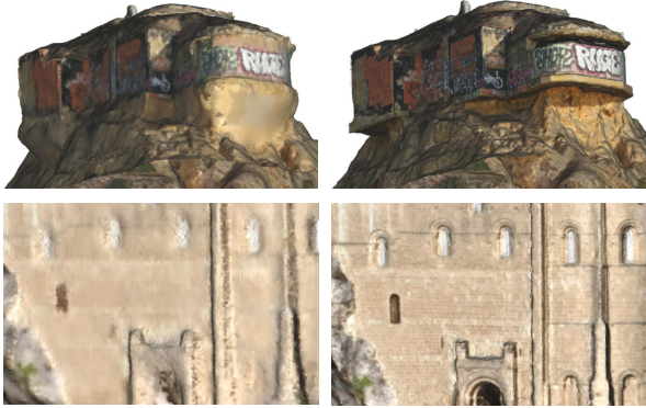
Fig. 7: Comparison of the coverage quality after the reconnaissance flight (left) and the successive flights (right). Occluded regions under the Bunker are not reconstructed (up). In addition, even though vertical surfaces such as Loarre's walls are covered, their observation yields poor scene reconstructions (down).
