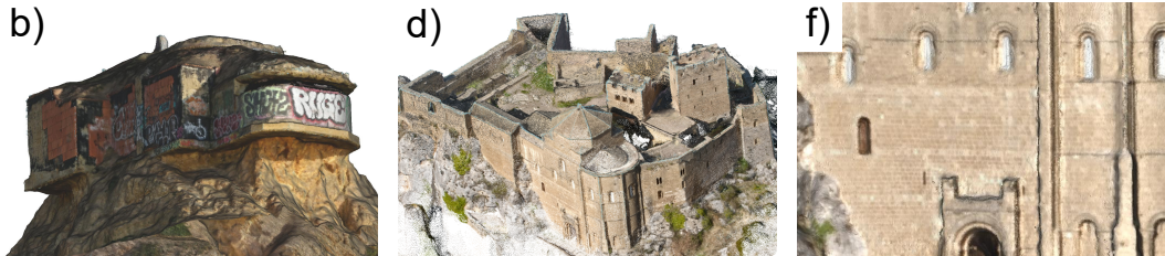
Figure 5.4: Comparison of the coverage quality after the reconnaissance flight (up) and the successive flights (down). Occluded regions under the Bunker are not reconstructed (a-b). In addition, even though vertical surfaces such as Loarre's walls are covered, their observation yields poor scene reconstructions (c-f).
