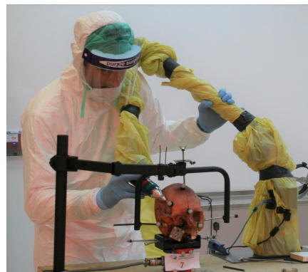
FIGURE 2.6: Measurement of the 3D coordinates of anatomical landmarks and Vicon markers with FaroArm to create the local coordinates systems of the skull, atlas, and axis.
