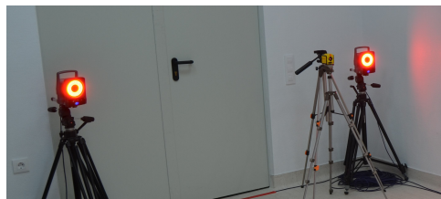
FIGURE 2.4: Two Vicon cameras (of a total of four), and one red-light laser, which was used as the reference for the initial position (neutral position) before all the movements.
